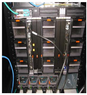
3) Connect one end of the second stacking module cable to switch A1 XG2 slot in Bay 1.
