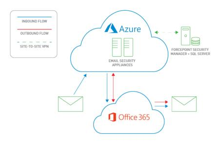
The Forcepoint Email Security Hybrid Module is an optional subscription that adds support for email hybrid service inbound pre-filtering in the cloud. See Email hybrid service configuration. The following diagram displays the workflow of Forcepoint Email Security and Forcepoint Security Manager in Azure with the addition of the Forcepoint Email Security Hybrid Module.
