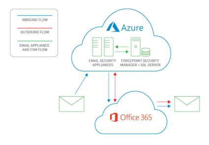
The following image displays Forcepoint Email Security deployed in Azure while Forcepoint Security Manager remains on-premises. This is the only deployment available for version 8.5, and is an additional option for versions 8.5.3, 8.5.4, and 8.5.5. The diagram depicts both inbound (blue) and outbound (orange) message directions.
