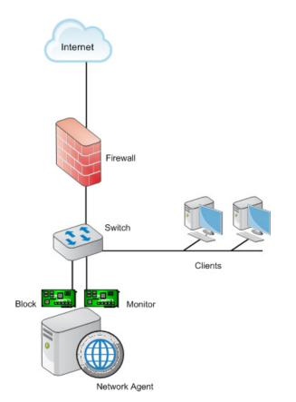
Install and configure each NIC before installing Network Agent:
