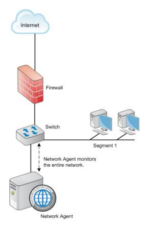
Optionally, deploy multiple Network Agent instances, with each instance monitoring a different segment of the network. This may be necessary in a busy network.
